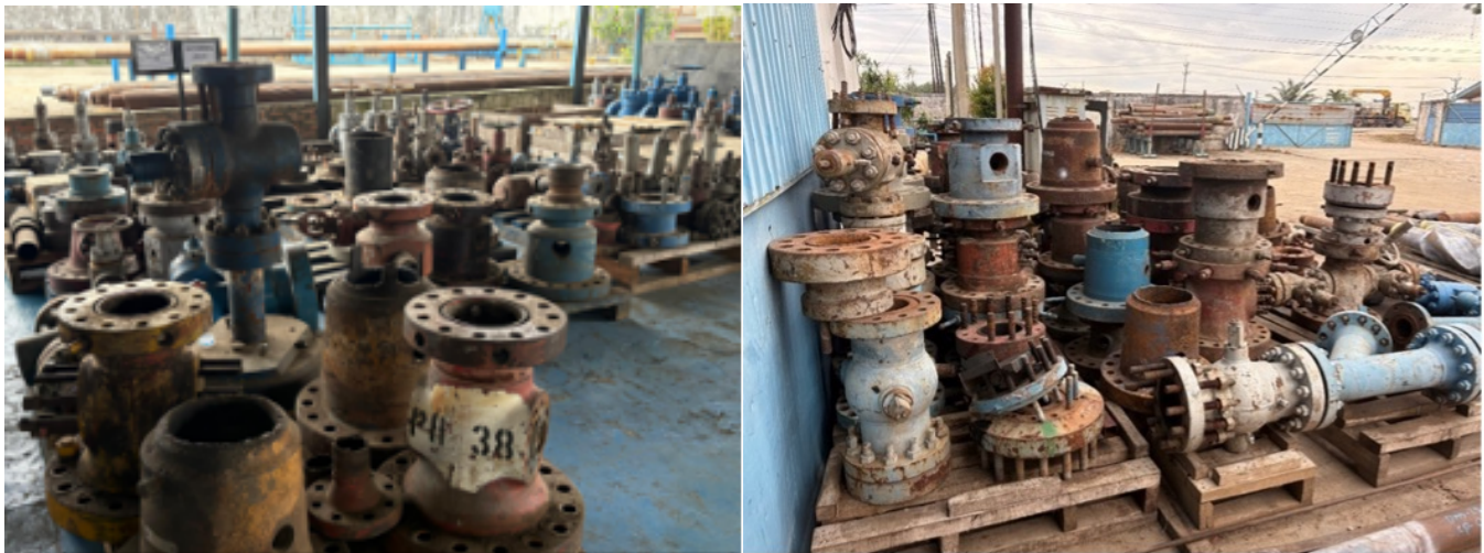
Used Wellheads Before Refurbishment
